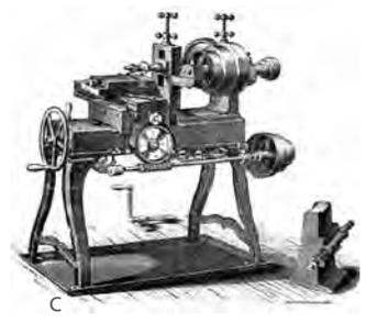
Three of the innovative firearms manufacturing machines developed for the Colt Armory. A) multiple-spindle vertical barrel boring machine; B) double-head face-milling machine; C) Lincoln miller. *From Tenth Census of the United States (1880): Manufactures, Vol. 2, 1883.*
